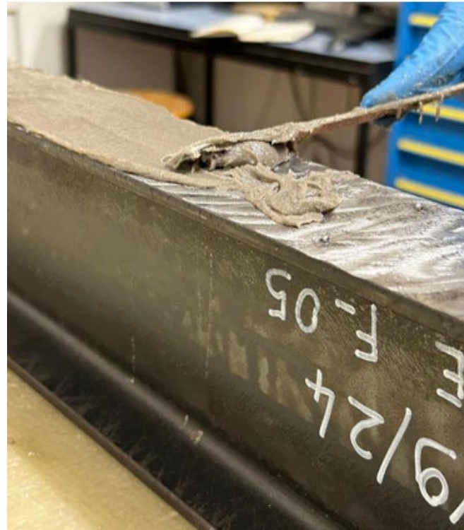
Application of a 2 mm adhesive layer
