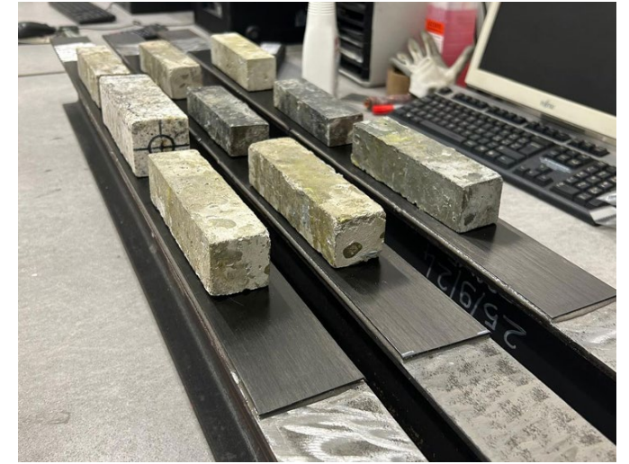
CFRP bonding and curing
